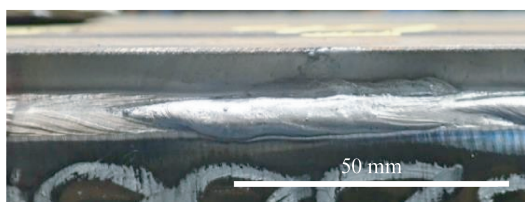
(a) Appearance of weld bead surface
